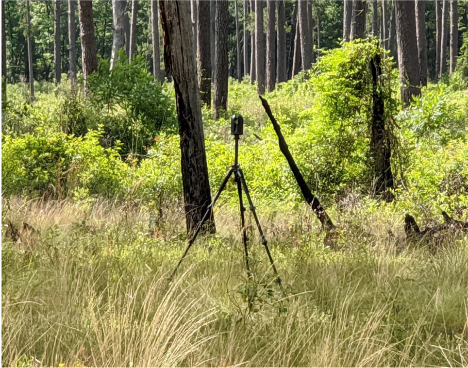
Fig. 1. The Leica BLK360 is lightweight and easy to deploy in the field. Its ease of use allows for rapid, unbiased data collection.
