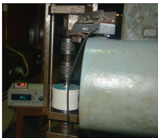
Figure 2: Standardization of Gnathodynamometer and load cell in the permanent lab of National Test House, Government of India
