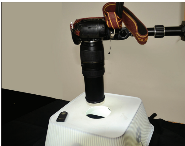
Figure 3: Self-made still photography setup for color evaluation
