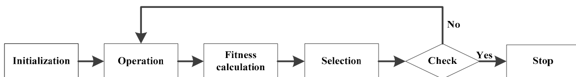
Figure 1. Optimization algorithm with evolutionary algorithms (EAs) as the optimization engine.
