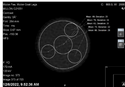
Fig. 3. DICOM images with HU values of phantom tubes (K 2 HPO 4 solution with concentration: 50 mg/cc).
