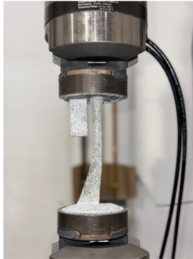
Fig. 9. 3D printed part encased in PMMA and prepared for DIC measurement.
