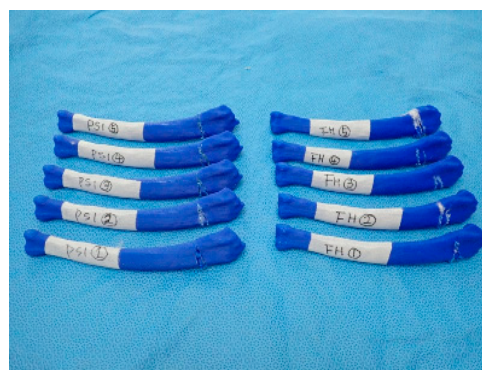
Figure 10. Simulative osteotomy result on phantom bone models. Patient-specific instrumentation (PSI) and freehand (FH) marked rapid prototyping bone models are the result of the osteotomy using the PSI and freehand, respectively. This picture was taken after the ex-vivo osteotomies were performed on the phantom bone models and the outer materials were removed.
