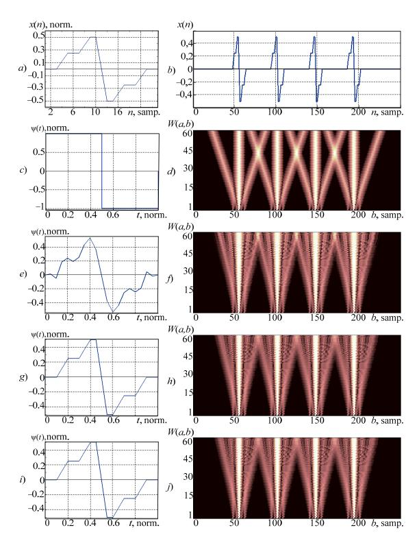
Figure 4. Results of research on synthesized wavelets: (a) the sample; (b) the analyzed signal; (c) the Haar wavelet; and the wavelet-spectrogram (d) that was obtained with its application; (e,g,i) the wavelets, obtained on the basis of polynomial, neural network, and spline models, respectively (before normalization); (f,h,j) wavelet-spectrograms obtained using synthesized wavelets (e,g,i), respectively.
