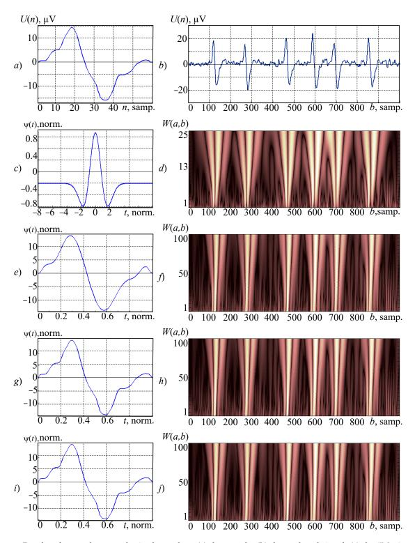
Figure 2. Results of research on synthesized wavelets: (a) the sample; (b) the analyzed signal; (c) the "Mexican hat" wavelet; the wavelet-spectrogram (d) that was obtained with its application; (e,g,i) the wavelets, obtained on the basis of polynomial, neural network, and spline models, respectively (before normalization); (f,h,j) wavelet-spectrograms obtained using synthesized wavelets (e,g,i), respectively.
