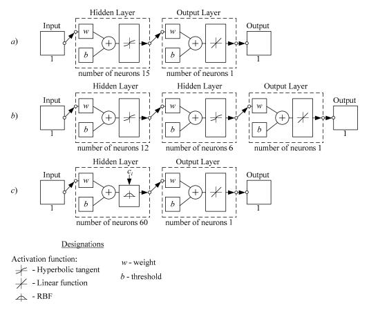
**Figure 3.** Artificial neural networks: multi-layer perceptron with one hidden layer (**a**), multi-layer perceptron with two hidden layers (**b**) RBF-network (**c**).
