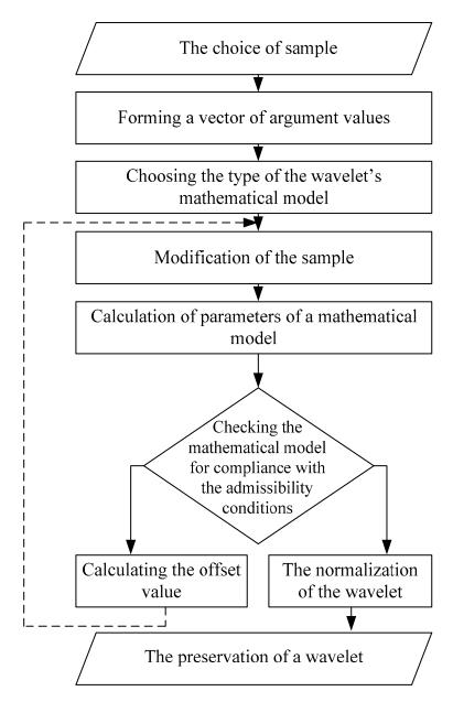
Figure 1. Modified wavelet synthesis algorithm for continuous wavelet transform of signals.
