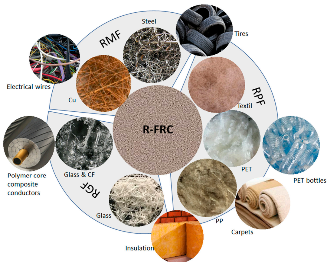
Figure 1. Types of recycled fibers used in R-FRC: recycled metallic fibers (RMF), recycled glass fibers (RGF), carbon fibers (CF) and recycled synthetic polymeric fibers (RPF).
