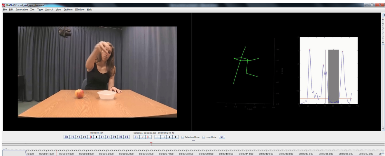
Fig. 4 Example of a video and kinematic pairing in ELAN. On the left, the standard video recording is being played, while on the right a skeleton of the motion capture data as well as the velocity profile of the right hand
