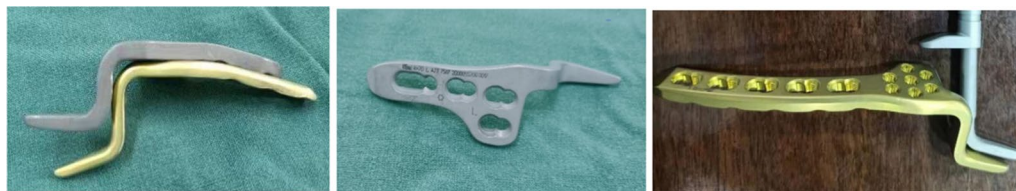
Fig. 2 In the past, the end hole of the hook steel plate was a 3.5 mm joint hole, but now it is changed to seven 2.7 mm universal holes. The hook angle of the hook steel plate in the past was 90°, and now a 110° steel plate is added
