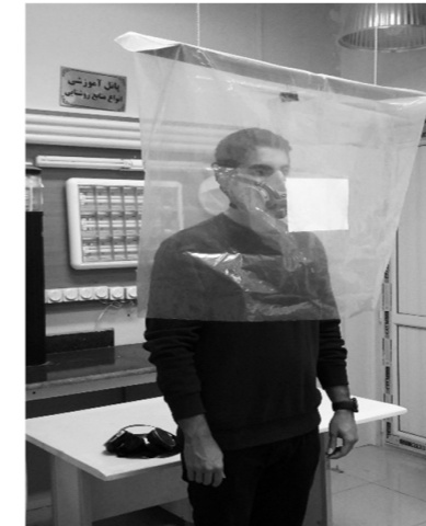
Fig. 1. The participant was inside the test hood during the IAA fit testing procedure.
