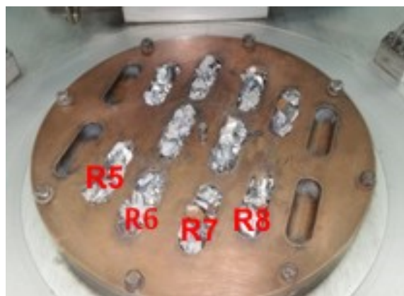
Figure 1. Metallic raw materials placed on the copper plate of VAR equipment.
