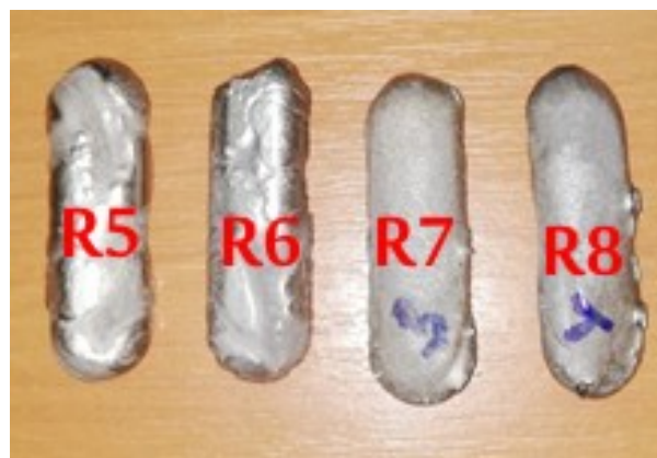
Figure 2. Mini-ingots of the alloys from TiMoZrTaSi system.
