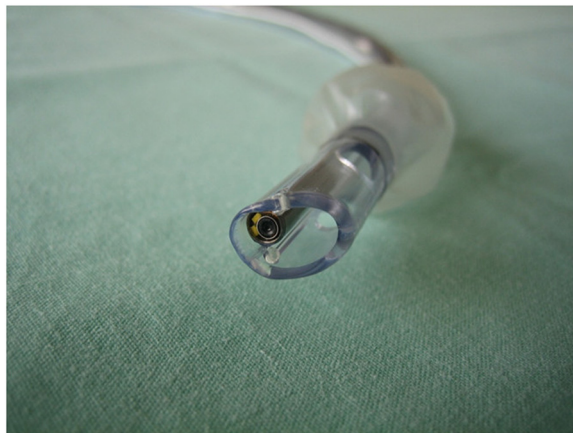
Figure 1 The VivaSight™ Single Lumen endotracheal tube with a camera embedded in its tip.
