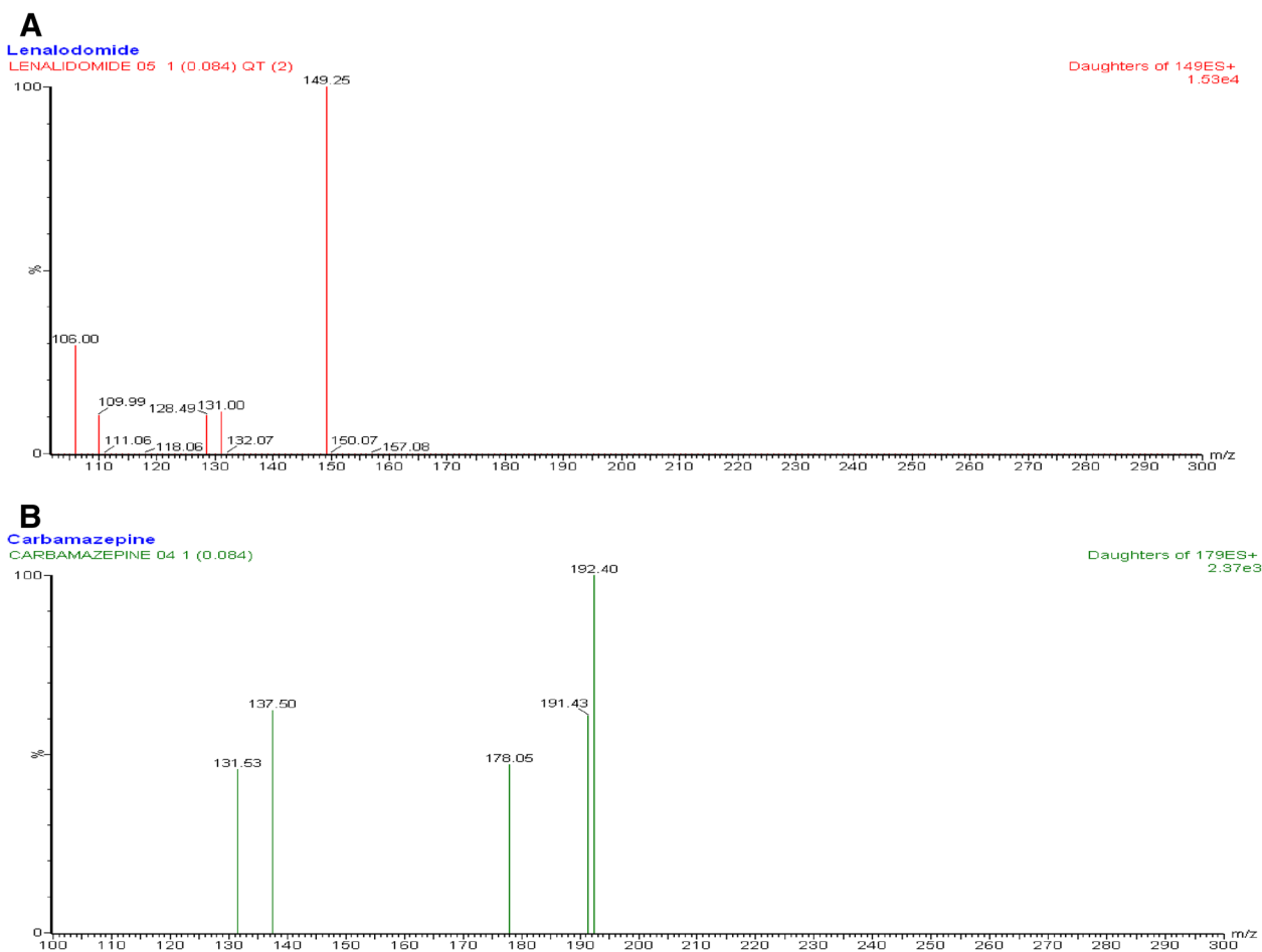
Figure 2 The product ion spectra of lenalidomide [A] and carbamazepine (IS) [B].
