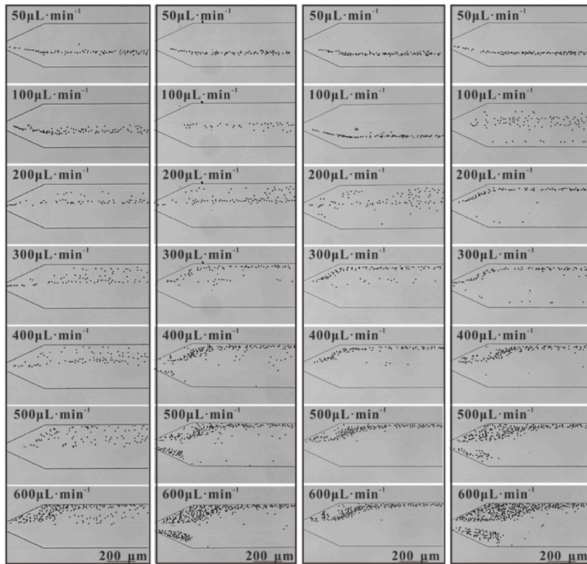
(a) Sharp cornerstructure (b) Arc-shaped structure (c) Semicircular structure (d) Rectangular structure
