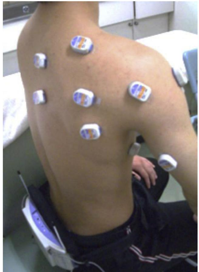
**Figure 1** Compact electrode telemeter system integrated into a wireless transmitter.
