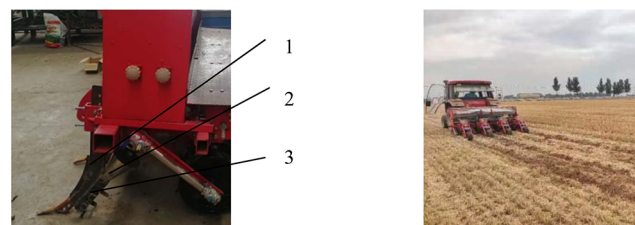
1. Deep loosening shovel 2. Fertilizer equalization and mixing device 3. Fertilizer guide box
