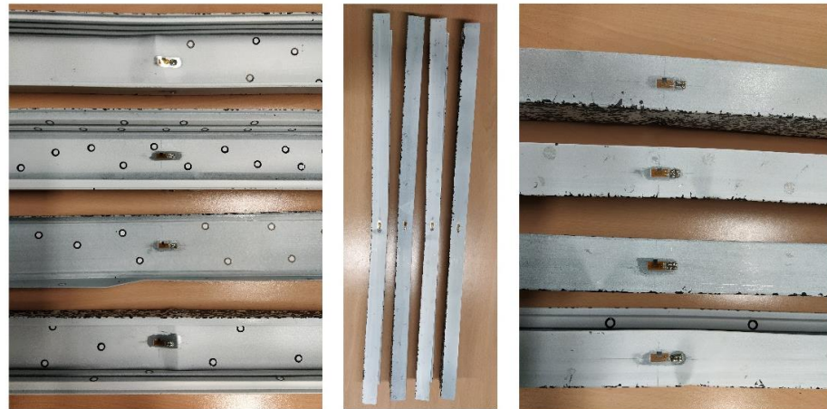
Figure 16. Mechanisms of failure of tested columns.
