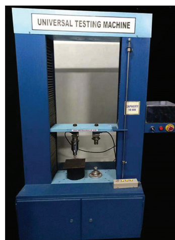
Figure 4: Universal testing machine used to measure load-bearing capacity for polyether ether ketone fixed dental prosthesis
