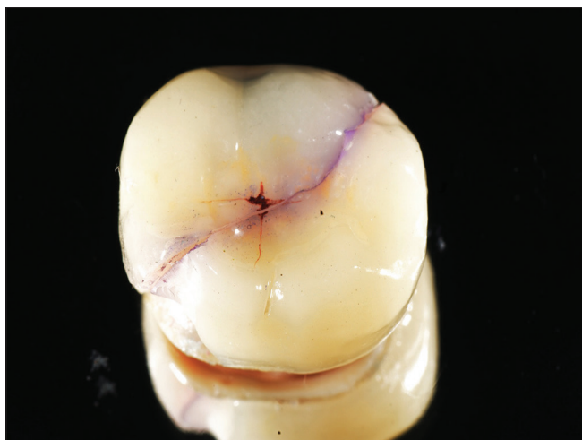
Figure 7: After fracture load measurements. Adhesive failures between polyether ether ketone framework and veneering lithium di-silicate
