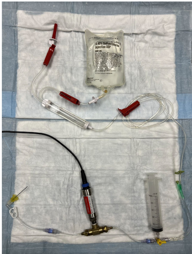
FIGURE 1 Line set-up for demonstration only. A 60 mL syringe (right) attached to intravenous line via three-way stopcock, with in-line pressure monitor (center).
