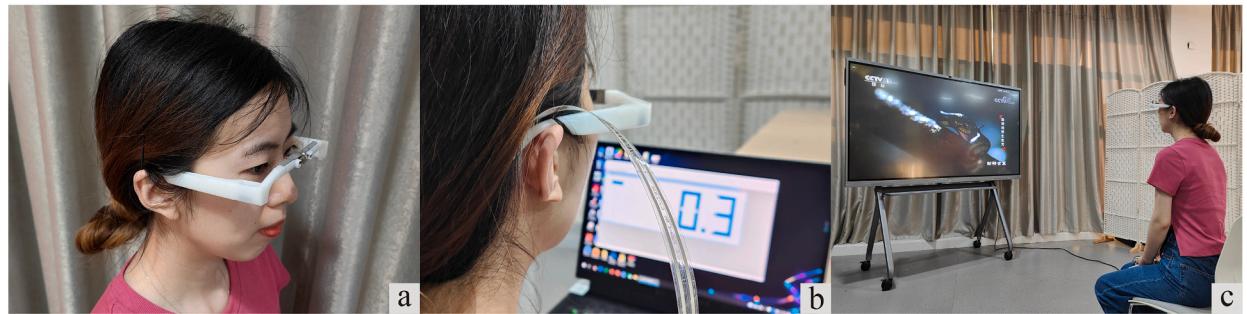
Fig. 3. Test procedure for (a) prototype wearing, (b) pressure measurement and (c) video viewing.
