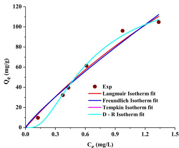
**Figure 5.** Isotherm fits for the adsorption of AB-25 removal by Cs-Trp@Fe<sub>3</sub>O<sub>4</sub>.
