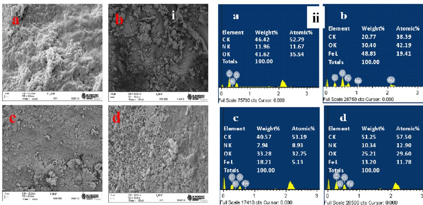
Figure 1. (i) SEM images and (ii) EDX and elemental analyses of: (a) Cs, (b) Fe<sub>3</sub>O<sub>4</sub>, (c) Tp@Fe<sub>3</sub>O<sub>4</sub>, and (d) Cs-Trp@Fe<sub>3</sub>O<sub>4</sub>.
