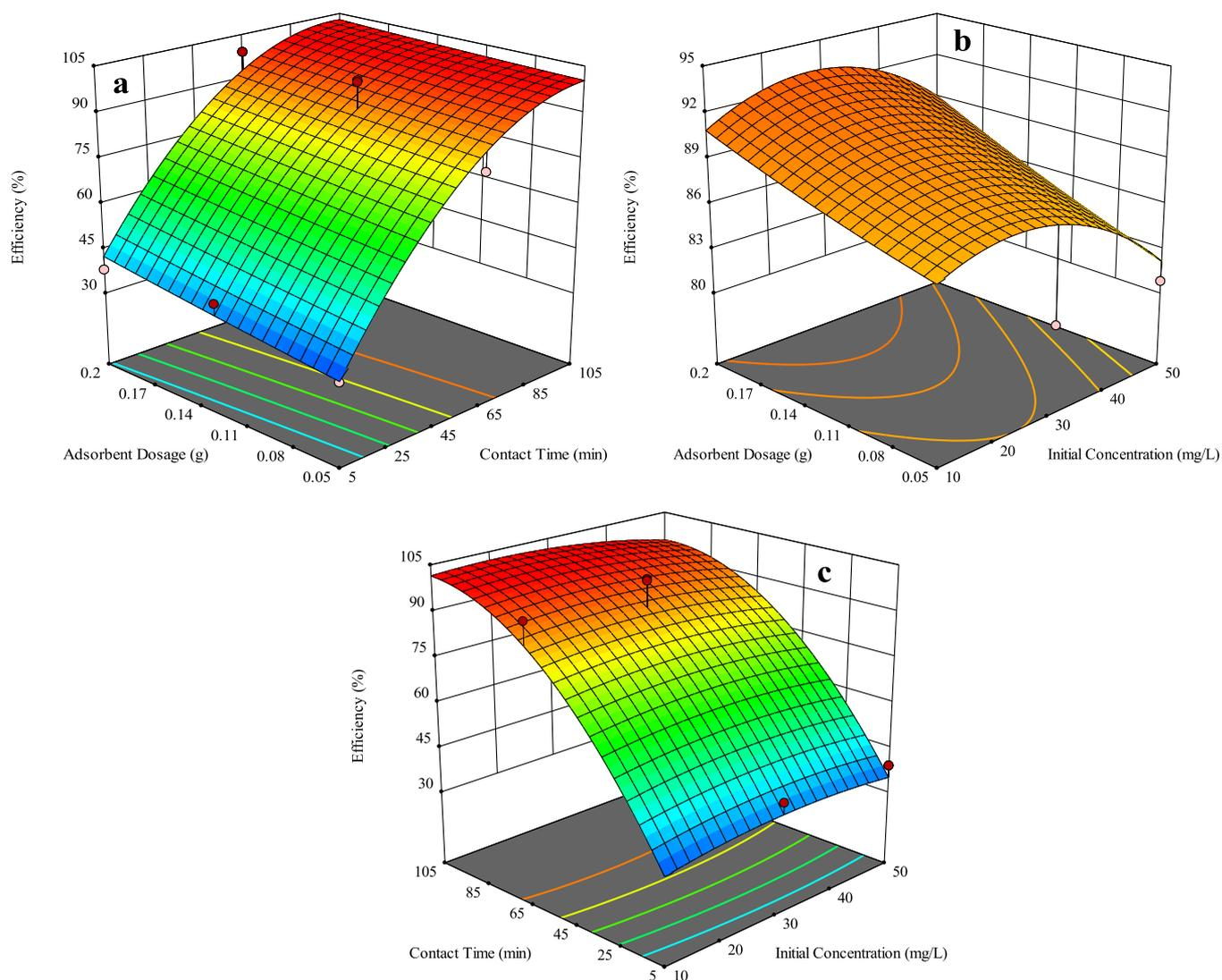
**Figure 6.** Response surface plot of the effect of (a) adsorbent dosage and contact time, (b) adsorbent dosage and initial concentration, and (c) contact time and adsorbent dosage on the removal efficiencies of the AB-25 dye by Cs-Trp@Fe<sub>3</sub>O<sub>4</sub>.
