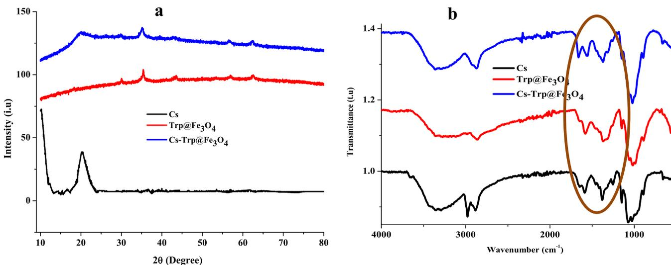
Figure 2. (a) XRD patterns and (b) FTIR spectra of chitosan, Tp@Fe<sub>3</sub>O<sub>4</sub>, and Cs-Trp@Fe<sub>3</sub>O<sub>4</sub>.
