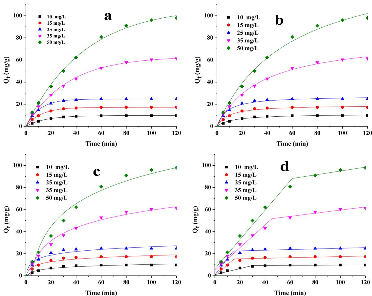
**Figure 3.** Kinetic model fits for the removal of AB-25 by Cs–Tp@Fe<sub>3</sub>O<sub>4</sub>: (a) pseudo-first-order, (b) pseudo-second-order, (c) Elovich, and (d) intra particle diffusion for different initial concentrations of AB-25.
