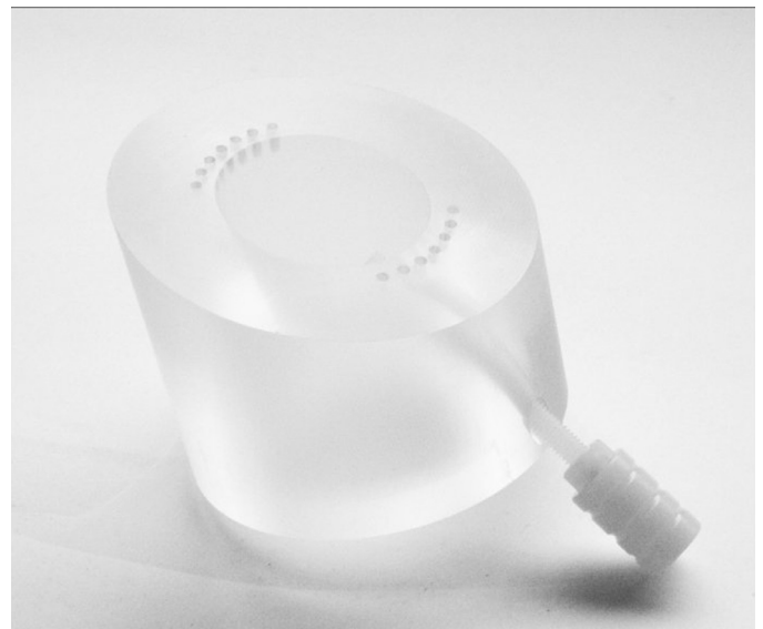
Fig. 6. Holes on the inner cylinder face enabled the cup to be pinned at different internal/external rotations.
