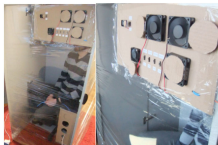
Figure 3. Left 2 fans ON~250 lpm Right 4 fans ON~1250 lpm.
