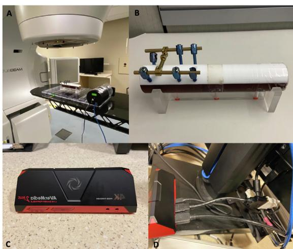
**Figure 2** Set-up of the simulated treatment with the QUASAR motion platform beneath the spine hardware phantom. 4K pass-through capture card was connected to the treatment console to achieve a high-definition recording of the simulated treatment.
