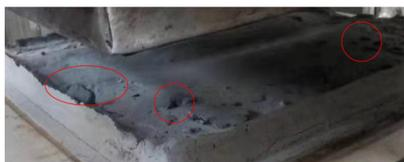
**Figure 10.** Local breakdown and short circuit of the fly ash filter cake layer during the leaching process.
