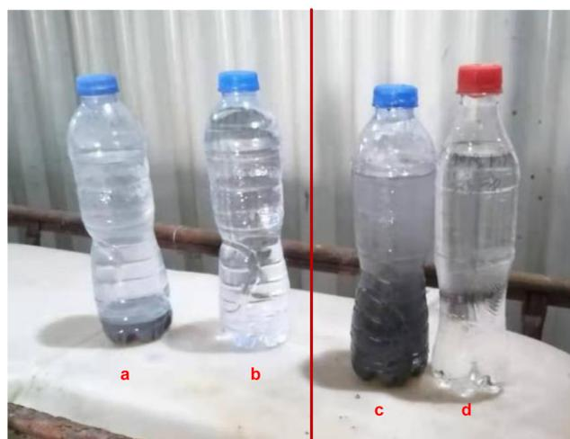
**Figure 9.** Comparison of the washing filtrate of two washing dechlorination processes. (a,c) Actual operating washing filtrate, and (b,d) test washing filtrate of the cyclic gradient washing dechlorination process. (a,b) States of still standing for 1 h; (c,d) states without still standing.
