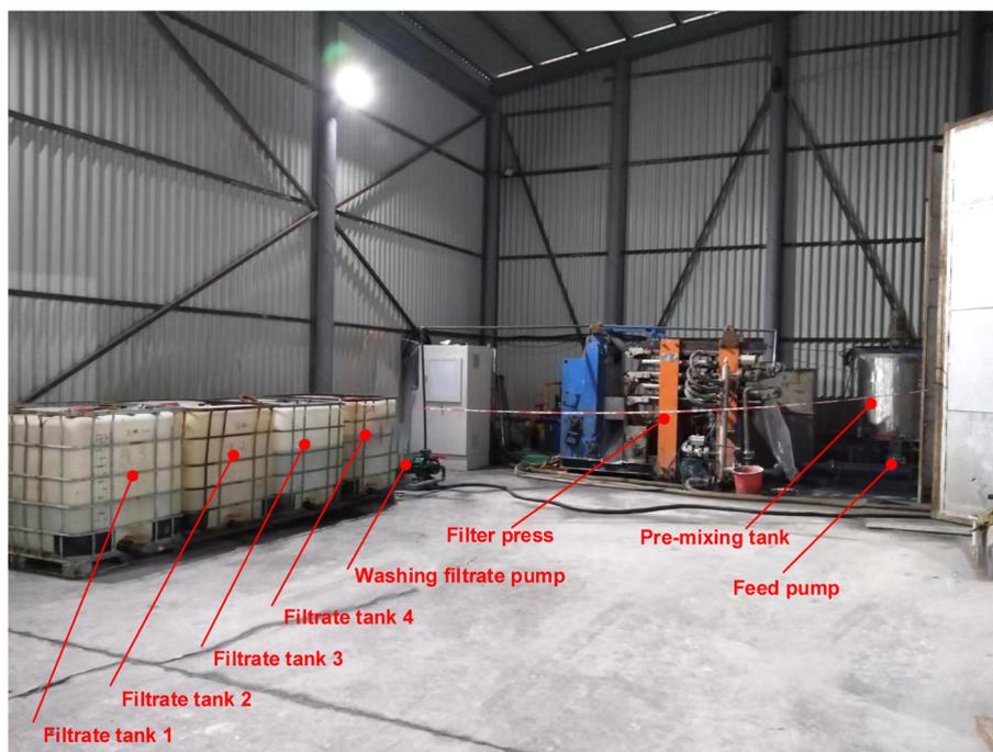
**Figure 4.** Fly ash cycle gradient water washing dechlorination system filter press.
