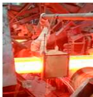
Figure 9. The MIT system in continuous casting set up.
