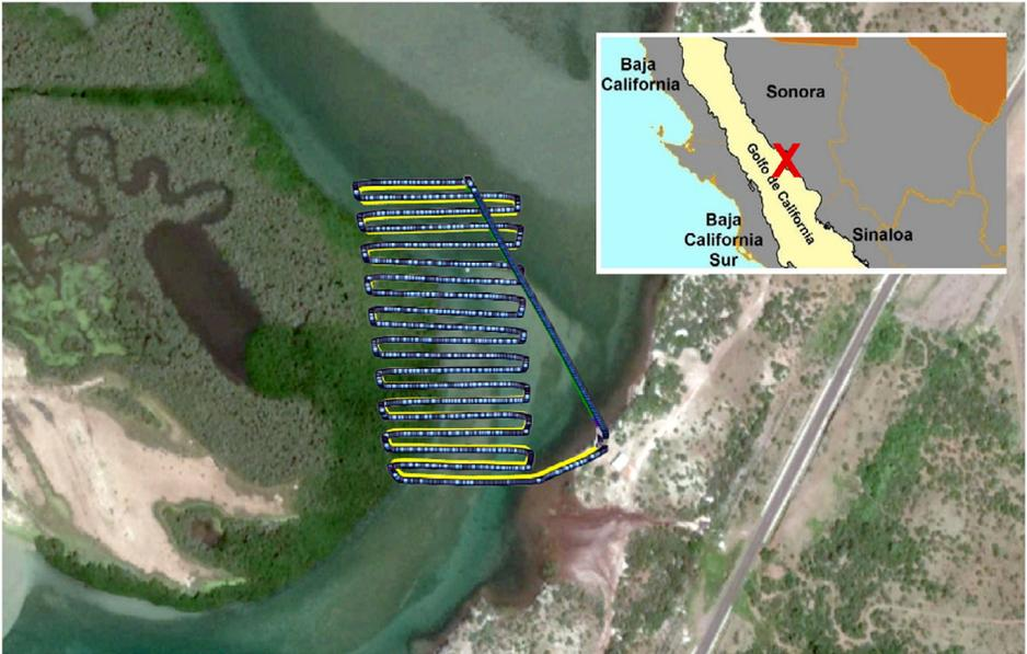
**Fig. 1.** Sky view of the coastal strip surveyed within “El Soldado” estuary, in Guaymas, Sonora. The yellow line identifies the flight path followed by the UAV. The blue dots on the yellow line are the images taken using a commercial-grade digital camera. Upper-right figure shows the location of the study site within a regional domain in Northwestern, México.
