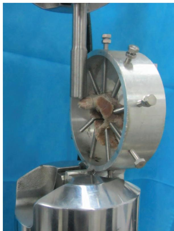
**Figure 3.** Testing of shear stiffness.
