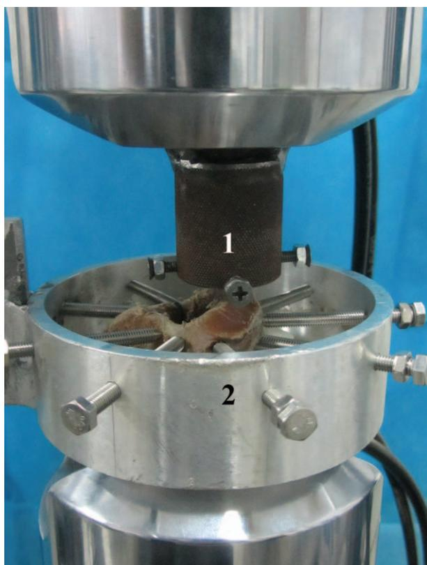
**Figure 2.** Testing of torsional stiffness and tensile stiffness. (1) The ferruginous ring equipped with 4 threaded positioning rods. Each rod was partially sharpened at the tip to securely fix the odontoid process. (2) An aluminum alloy ring with 9 threaded positioning rods designed to securely fix the body of the C2 vertebrae.
