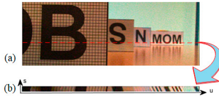
Figure 2. An example of an EPI. (a) is a central view image, (b) is an EPI corresponds to the row of the red dotted line in (a).
