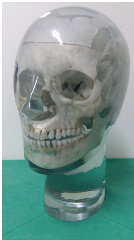
Fig. 3. A real skull phantom with a soft-tissue replica.
