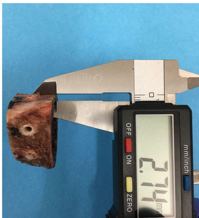
Figure 4. Measuring cortical thickness of juvenile bovine sample.
