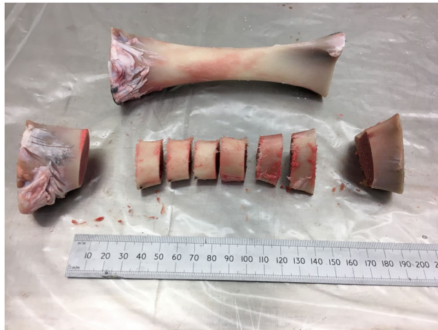
Figure 1. Sectioning of long bone diaphysis, with six cut diaphyseal samples retained for testing.
