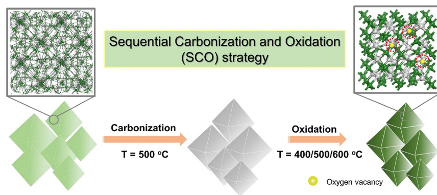
Figure 14. Fabrication procedure of SCO-derived Cr 2 O 3 catalyst
