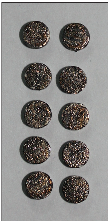
Figure 2: Laser surface-modified and conditioned titanium zirconium samples
