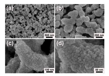
**Figure 2.** The differently magnified field emission scanning electron microscope (FESEM) images of porous worm-like Au synthesized in the presence of  $[N_{3333}]$ [Gly]: (**a**) 20,000 times, (**b**) 50,000 times, (**c**) 100,000 times and (**d**) 200,000 times.
