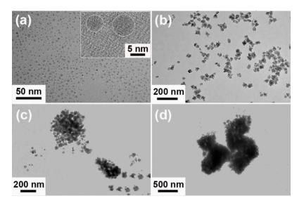
**Figure 8.** TEM images of as-synthesized Au products assisted by [N<sub>3333</sub>][Gly] at different interval: (**a**) 3 min, (**b**) 10 min, (**c**) 4 h, and (**d**) 8 h; the inset of (**a**) shows the magnified TEM image.
