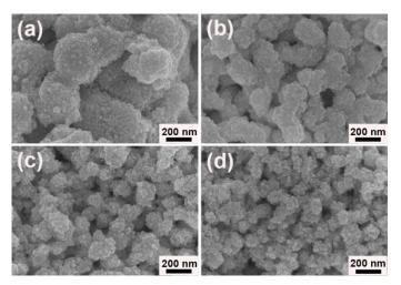
**Figure 7.** FESEM images of as-prepared Au samples assisted by  $[N_{3333}]$ [Gly] at different temperatures: (a) 7 °C, (b) 40 °C, (c) 60 °C, and (d) 80 °C.
