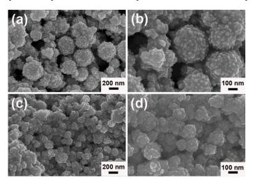
**Figure 5.** FESEM images of as-prepared Au samples assisted by different ILs: (**a**,**b**) [N<sub>1111</sub>][Gly], and (**c**,**d**) [N<sub>4444</sub>][Gly].
