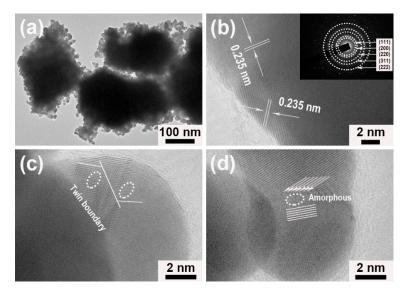
**Figure 3.** Porous Au worms synthesized in the presence of [N<sub>3333</sub>][Gly]: (**a**) transmission electron microscope (TEM) image, and (**b**–**d**) high resolution transmission electron microscope (HRTEM) images; the selected area electron diffraction (SAED) pattern is presented in the inset of (**b**).
