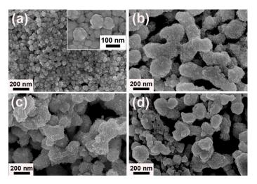
**Figure 6.** FESEM images of as-prepared Au samples assisted by [N<sub>3333</sub>][Gly] with various concentrations: (**a**) 50 mM, (**b**)100 mM, (**c**) 150 mM, and (**d**) 200 mM; the inset of (**a**) shows the magnified SEM image.
