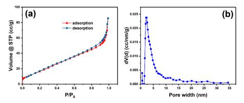
Figure 4. N<sub>2</sub> adsorption-desorption isotherms (a) and porous size distribution (b) of porous Au worms.
