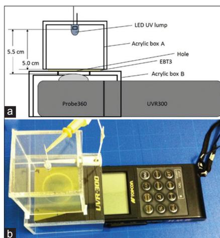
**Figure 1:** Ultraviolet-A rays emitted from the light-emitting diodes pass through the Gafchromic EBT3 film and reach the ultraviolet meter. (a) Arrangement of the ultraviolet light-emitting diodes and ultraviolet measurement device (lateral view). The Gafchromic EBT3 film is placed between acrylic boxes A and B; (b) photograph of the measurement device and ultraviolet meter. The Gafchromic EBT3 film is taped to acrylic box B
