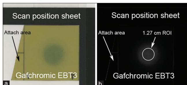
**Figure 2:** (a) Colored Gafchromic EBT3 film irradiated with 375-nm ultraviolet-A for up to 60 min and (b) subtraction image with region of interest indicated
