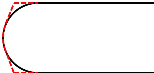
**FIGURE 1** Schematic highlighting the differences in how multi-leaf collimator leaf tips are modeled in the Monte Carlo framework (solid black line) versus the leaf-tip design used by the Varian Millennium 120 multi-leaf collimator (dashed red line). Leaf tips are not drawn to scale
