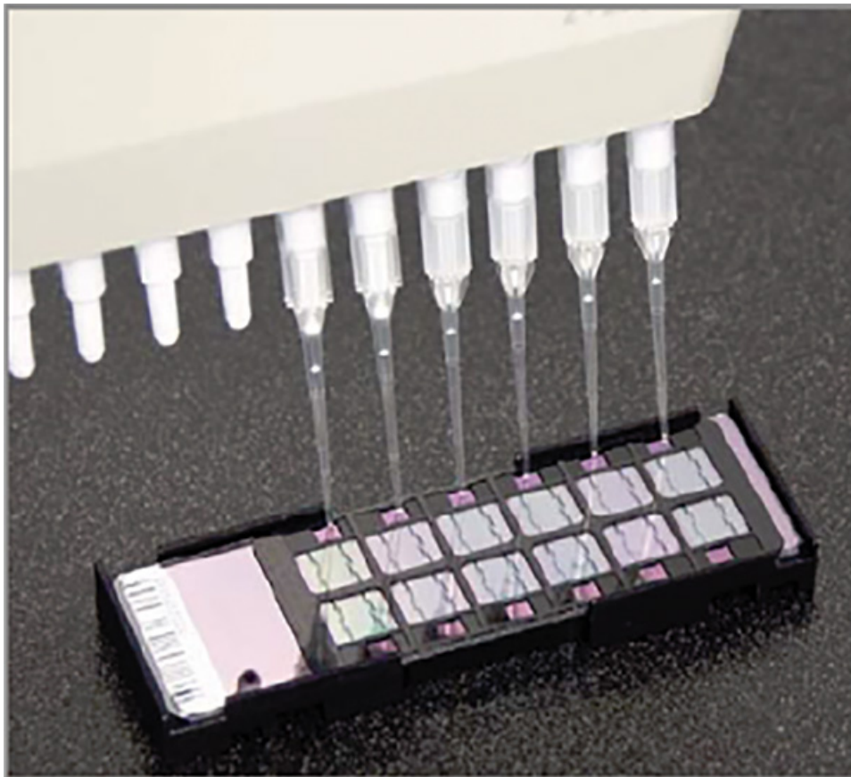
Figure 3. Loading a Beadchip – Dispense the sample on the inlet ports. [12] Click here to view larger image.
