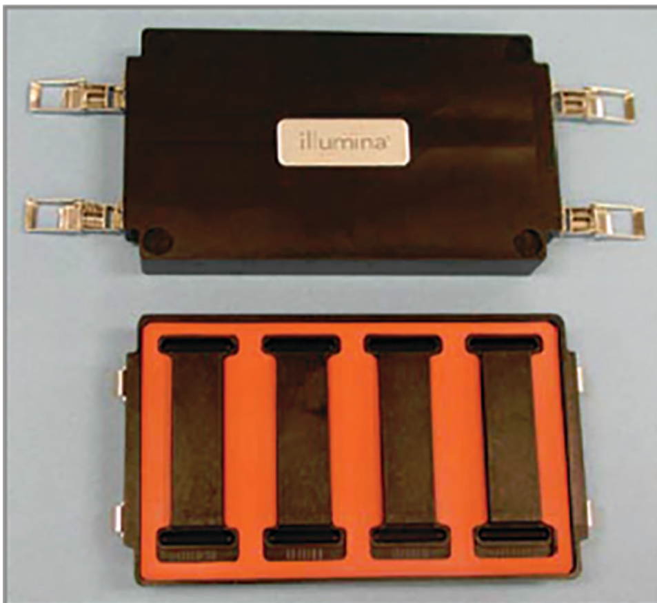
Figure 2. Complete Hyb Chamber base and mat, plus lid. [12] Click here to view larger image.
