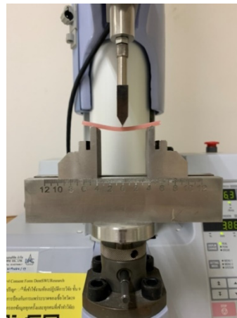
Figure 4. The testing machine and resin workpieces during the three-point flexure test.
