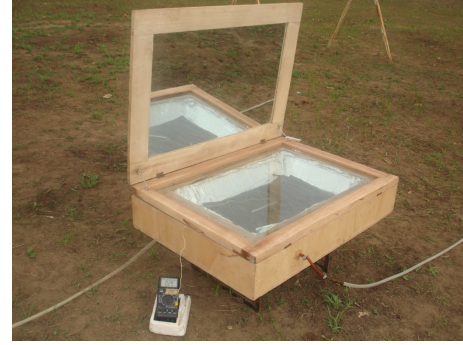
FIGURE 1: Experimental arrangement for temperature measurements (collector area, 0.47 \text{ m}^2 ).
