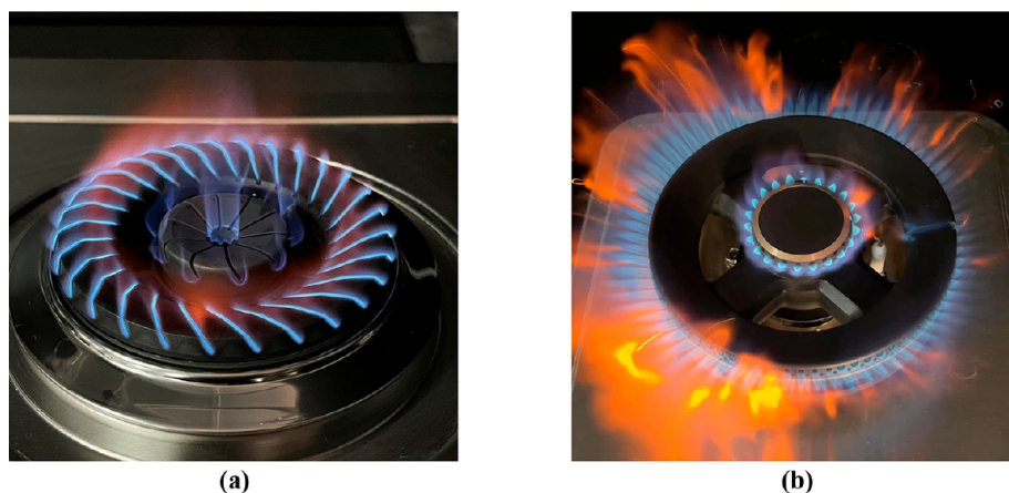
Figure 18. Destabilizing phenomena of flame: (a) blow-off; (b) flashback.
