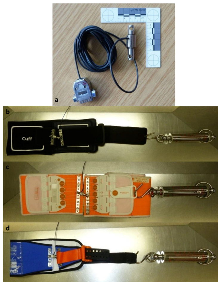
Figure 1. Used devices: (a) Newtonmeter; (b) Pneumatic pelvic sling VBM ® prepared with Newtonmeter and tension spring; (c) T-POD ® prepared with Newtonmeter and tension spring; (d) SAM Sling ® prepared with Newtonmeter and tension spring (source: Haussmann [22], modified).
