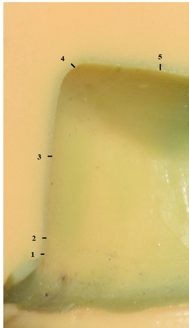
Fig. 2 Internal fit specimen. Silicon replica specimen with five reference points for surface quadrant.
