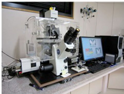
Fig. 1 Time-lapse cinematography (TLC). The inverted microscope was equipped with a CCD digital camera (Roper Scientific Photometrics, USA) connected to a computer, and images were displayed via MetaMorph (Universal Imaging Co., USA). Digital images of the
