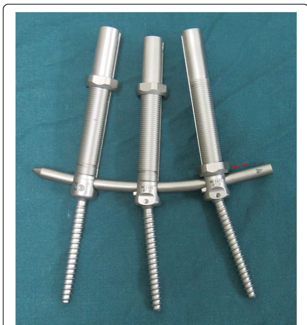
Fig. 1 The novel percutaneous self-expanding forceful reduction screw system presented is uniaxial screws with reduction angles and drop-prevention bolts (red arrow). From the left to right screws, the reduction angles are 0^\circ , 6^\circ , and 9^\circ in turn
