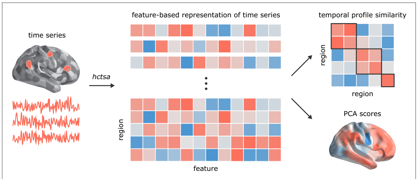
Figure 1. Temporal phenotyping of regional dynamics. The highly comparative time-series analysis toolbox, hctsa (Fulcher et al., 2013; Fulcher and Jones, 2017), was used to extract 6441 time-series features of the parcellated time-series for each brain region and participant, including measures of autocorrelation, variance, spectral power, entropy, etc. Regional time-series profiles were then entered into two types of analyses. In the first analysis, pairs of regional time-series feature vectors were correlated to generate a region \times region temporal profile similarity network. In the second analysis, principal component analysis (PCA) was performed to identify orthogonal linear combinations of time-series features that vary maximally across the cortex.
