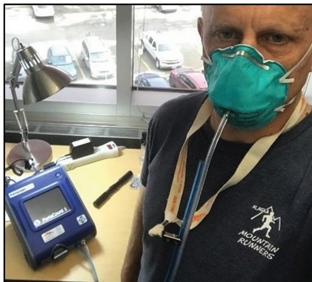
Figure 3. Fit test of N-95 respirator.
