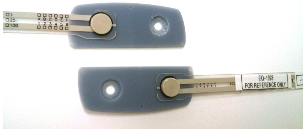
FIGURE 2: Modified, force-sensing lateral interbody cage
