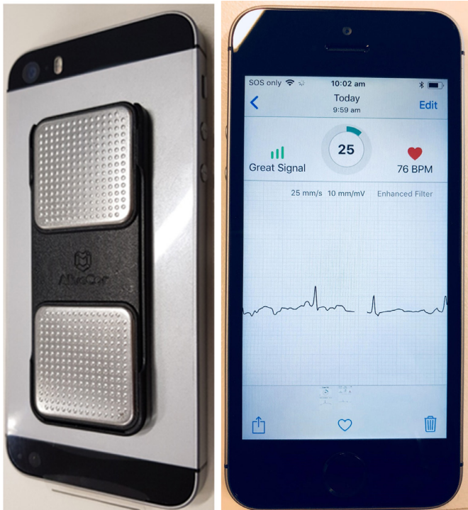
Figure 1 Kardia device and iECG reading.
