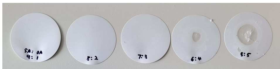
Figure 3 Filter papers showing a smear of oil droplets from the binary mixtures with oleic acid content above 30%.
